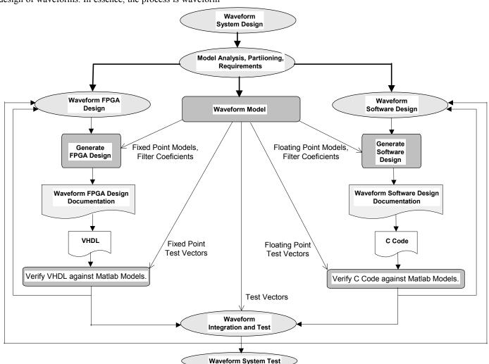
Figure 3. Rapid Waveform Modeling Applied to Software/FPGA Development Cycle.
