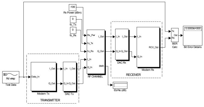
Figure 1. Waveform Model Components.
