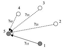
Figure 2 Propagation Losses to Node 5, the Node of Interest of Node 1
