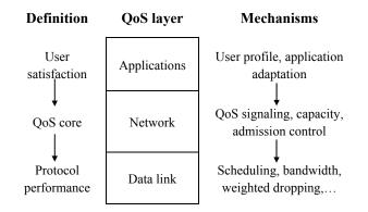
Figure 2. QoS layers, definitions and support mechanisms [2].
