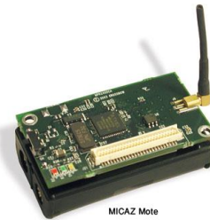
Figure 1 - The MicaZ Crossbow Berkeley Mote
