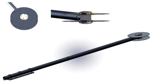
Figure 1: RHCP and LHCP GNSS antennas separated by two aluminum disks and mounted on a two meter pole. Cables leading to the antennas are inside the pole.
