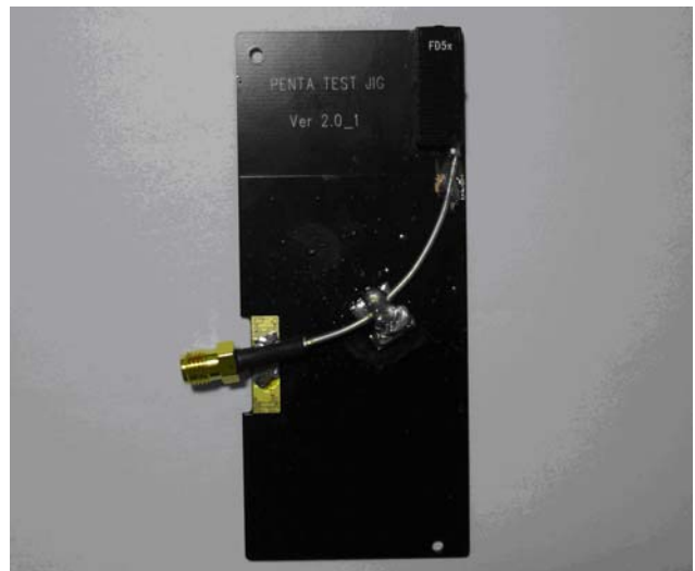
Fig. 5. Antenna mounted on the jig board
