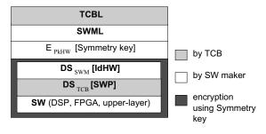
Figure 6: SW hybrid encryption
