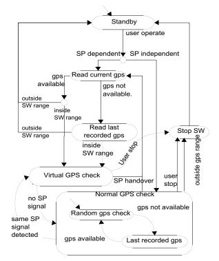
Figure 7: Stateflow of GPS checking scheme
